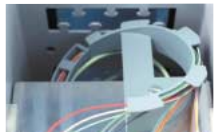
Security concept for fiber and cable protection: min. bending radius (40 mm) of pigtails guarantees optimum transmission. Loose tube protection at insertion in and removal from mounting channel. Mechanical protection is provided by lamella.
