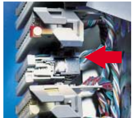
Full access for jumpering and testing Permanent protection of persons and equipment
